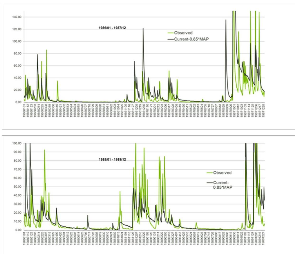
Figure 8-1: Typical correspondence of observed and simulated daily streamflows at W2H005 ( $\text{m}^3/\text{s}$ ) for two randomly selected years
