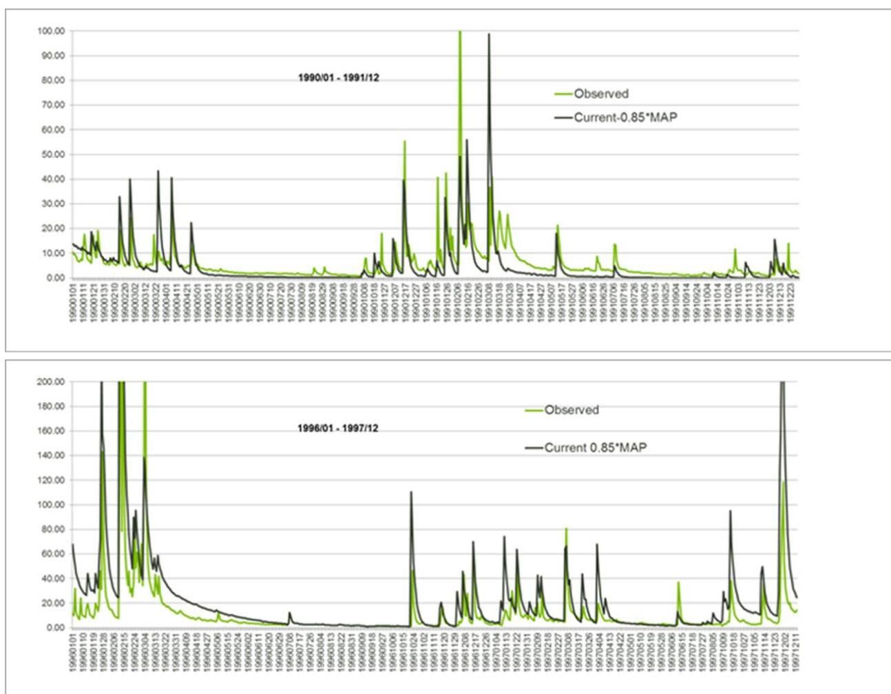
**Figure 6-1: Typical correspondence of observed and simulated daily streamflows at W2H006 (m<sup>3</sup>/s) for two randomly selected years**
